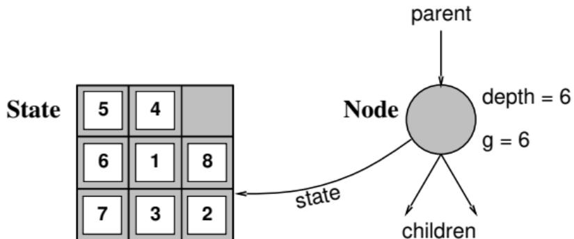
The Expand function creates new nodes, filling in the various fields and using the Operators (or SuccessorFn) of the problem to create the corresponding states.
