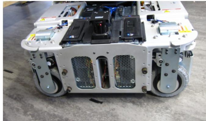
PR2: Double wheel construction to reduce friction while turning the wheel
